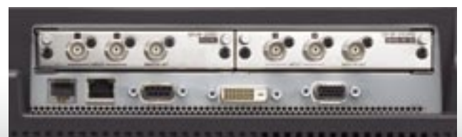
LMD-1750W Connector Panel and Option Slots
