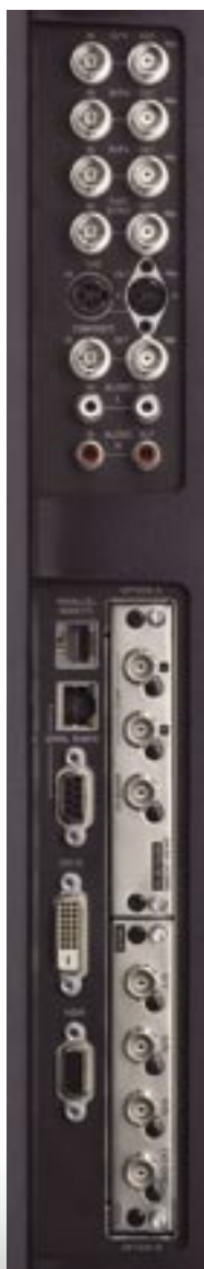
LMD-4250W Connector Panel and Option Slots
